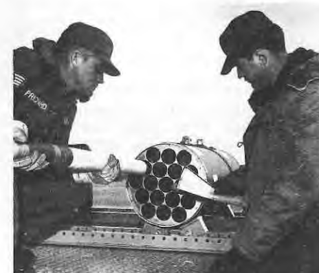
Air Force photo demonstrating how 2.75-inch rockets are loaded in 19-rocket pods ( Ordnance , Nov.-Dec. 1970)
