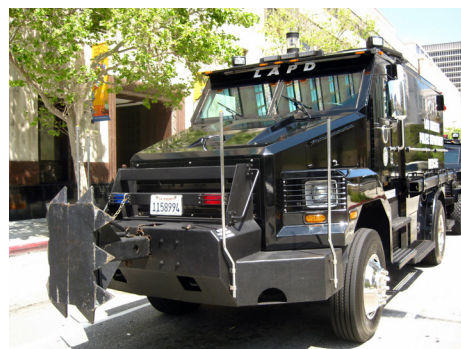
BEARCAT Los Angeles Police Department S.W.A.T. ‘Rescue 1’ B.E.A.R showing a battering ram attachment. Photo: Steve Devol/Wikicommons
